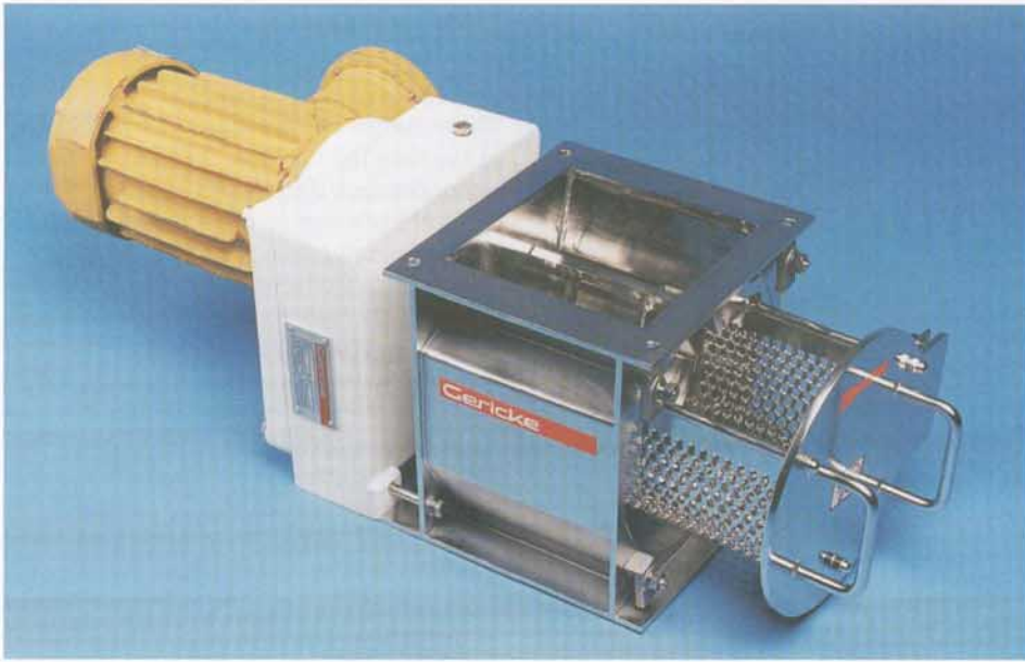
Fig. 2 NBS 200x200 Nibbler with screen: products pass vertically from the top of the machine to the bottom. Rotating paddles force the product through the hole in the screen or sieve.
