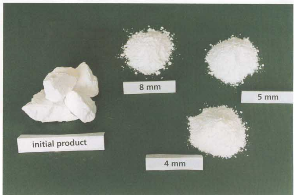
Fig. 1 The initial product, an organic salt, forms large lumps. They are reduced in the Nibbler to 8 mm, 4 mm or 5 mm, according to the screen that is used.
