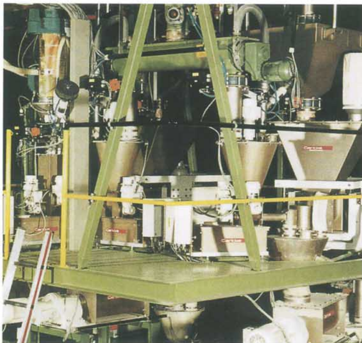
Eight ingredients are delivered by weigh feeders and two continuous mixers to a primary and side extruder.
