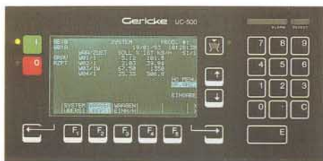
Example: System-control for 4 weigh feeders
