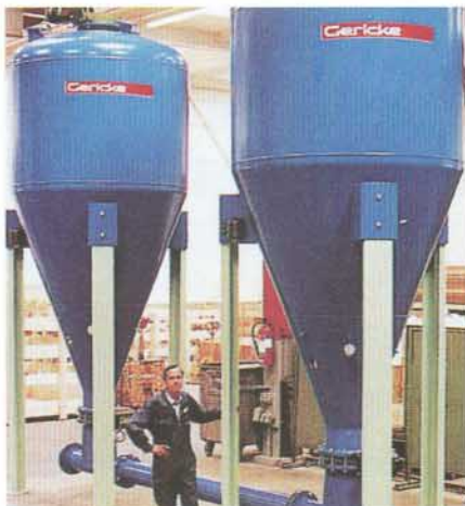
Fig. 3: Gericke twin vessel dense phase conveyor PHFD 5750
